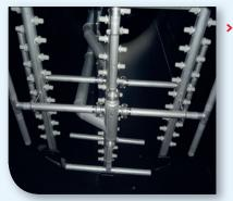
Specially designed resin collectors separate and transfer anion and interface resins to prevent mixing and contamination of the resin types.
